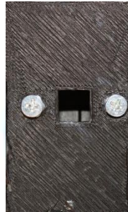
Figure 3. Image of the Optical input of the spectrometer
