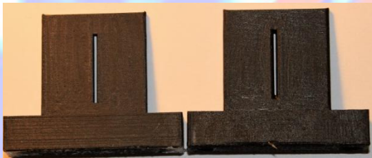
Figure 4. Image showing the 3D printed entrance slit and the current slit installed in the spectrometer.
