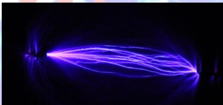
Figure 15 . Electric discharge generated by the bipolar Tesla coil.
