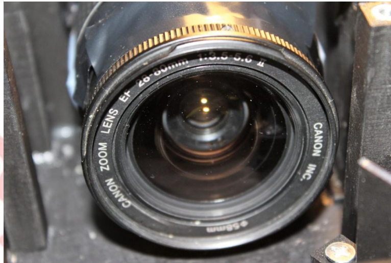
Figure 6. Image showing the focusing lens of the spectrometer.
