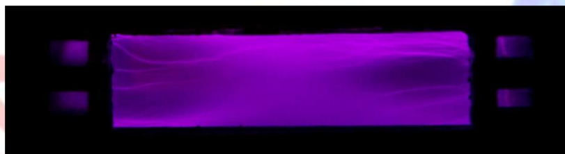
Figure 17. Plasma of pure Argon generated by the unit
