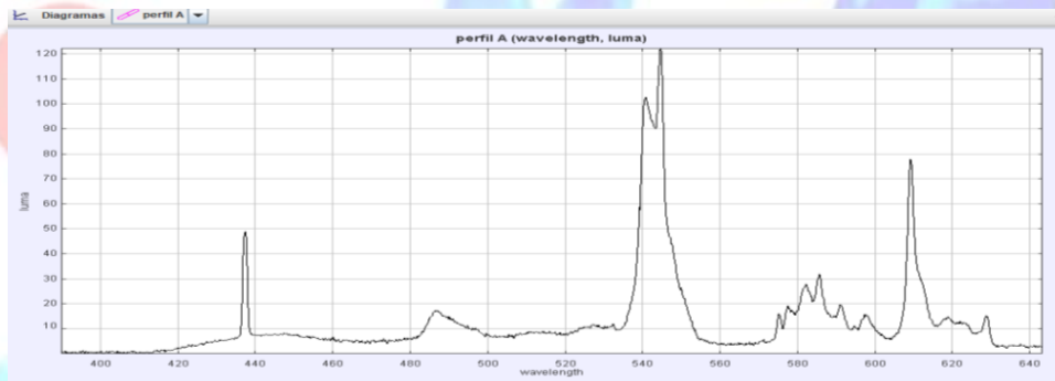
Figure 9. Spectrum of a compact fluorescent light source taken with the DIY spectrometer.
