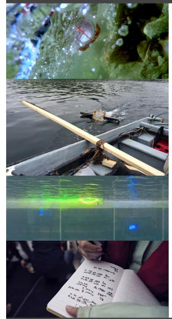
No matter where you use BabyLegs, the main issue is to make sure the mouth of the container stays at the surface of the water at all times, so most of the mouth is underwater, and a small amount is above water. This ensures the surface of the water, where most buoyant plastics are, is always entering the container.
