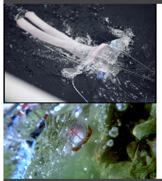
Created with baby's tights, soda pop bottles, and other inexpensive and easy to find materials, Babylegs can be used to skim the surface of water in rivers, streams, and oceans for floating marine microplastics by hand or from a boat. This instrument is called a **surface trawl**.
